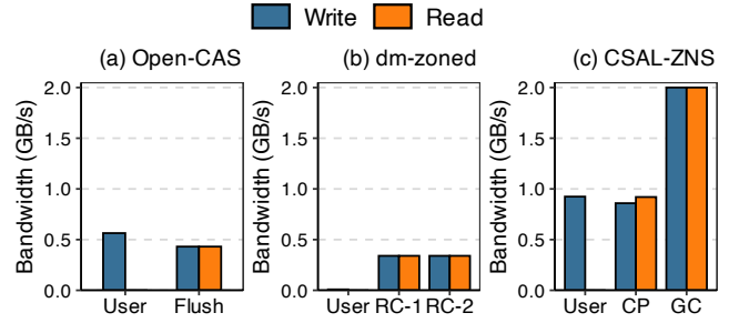
Figure 17. Backend Traffic under 64KB Random Writes. dm-zoned performs reclaiming from random to sequential zones (RC-1) and from sequential to random zones (RC-2). Open-CAS only performs flushing. CP and GC mean compaction and garbage collection.
